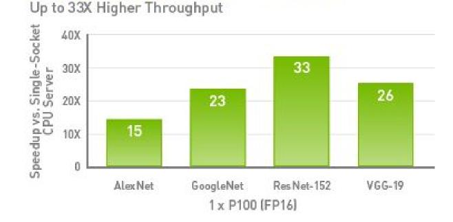
CPU Server: Single Xeon E5-2690 v4 @ 2.6GHz | GPU Servers: Single Xeon E5-2690 v4@2.6GHz with 1XP100 (PCle) | Ubuntu 14.04.5 | TensorRT 2.0 | CUDA 8.0.42 | cuDNN 6.0.5 | NCCL 1.6.1 | Batch size 128 | Precision FP32 (CPU) | FP16 (P100 GPU).
